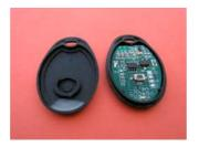
2. You will end up with 2 parts. One consisting of electronic component and second with rubber insert.
