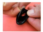
3. Remove rubbber insert from the shell.
